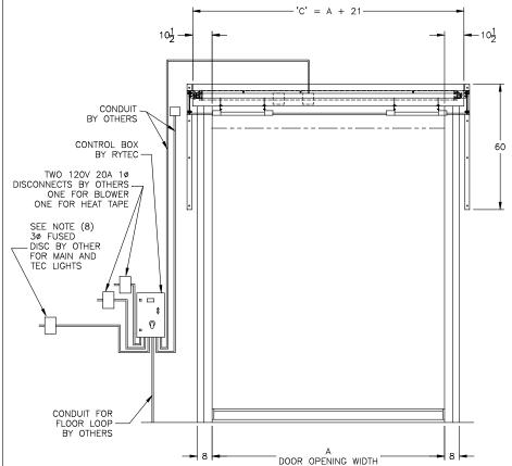
NOTES: RYTEC CORP. DOES NOT GUARANTEE A FROST FREE DOOR. THE RANGE OF THE TEC LIGHTS IS APPROXIMATELY TEN (10) VERTICAL FEET. DEPENDING ON SITE CONDITIONS AND RELATIVE HUMIDITY, IT IS POSSIBLE FOR FROST TO BUILD UP ON THE LOWER PORITION OF THE DOOR PANEL.
